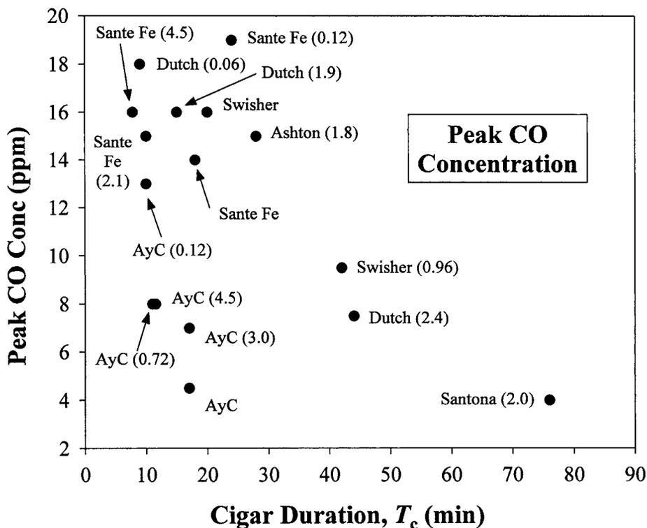
**Figure 4.** Plot of peak CO concentration versus cigar duration for 16 experiments where CO was measured. Each point is labeled with the cigar brand and the air exchange rate in units of air changes per hour (for experiments where the air exchange rate was determined). Notice that except for the AyC cigars, which have lower total emissions than most of the other cigars, there is a trend towards lower peak CO concentration as the cigar duration increases.
