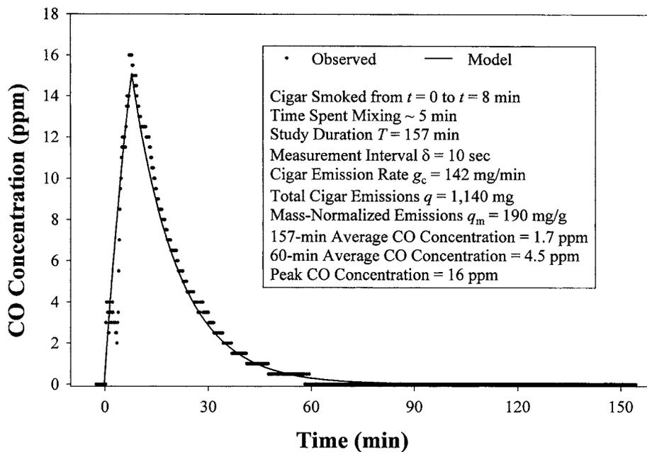
**Figure 2.** Observed CO concentrations and those predicted by a mass balance model during and after a cigar smoking experiment in a 49.6 m<sup>3</sup> office (experiment O-2). CO emission factors calculated using the model are shown.
