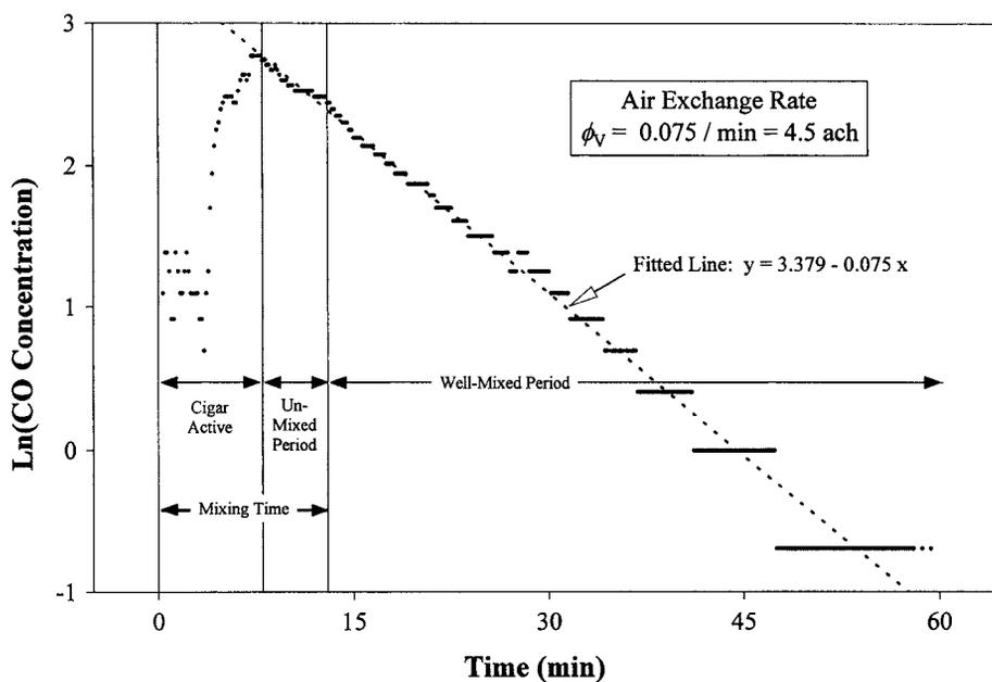
**Figure 1.** Experimental results from a cigar experiment in an office (experiment O-2) showing how the pollutant decay rate  $\phi$  is determined (in this case, for carbon monoxide). Notice that the unmixed time period (estimated at 5 min) is under 10% of the source-off time period, suggesting that the room can be considered to be well-mixed.
