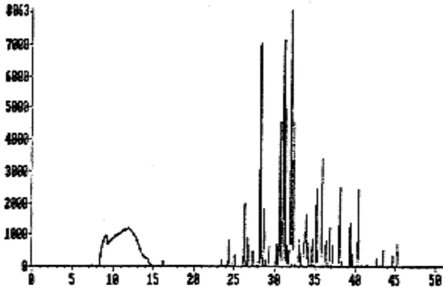
Figure 1. Reconstructed ion chromatogram of Headspace of liquid air freshener sampled directly (top) and by evacuated canister (bottom).
